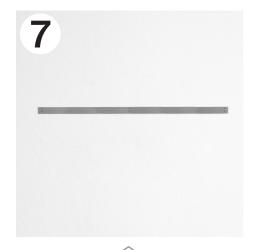
If several panels are to be installed side by side, we recommend the use of a longer suspension rail (2 m). This reduces the number of holes made in the wall and minimises installation time.
