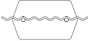
! Place the Mute panel correctly around the two tubes.
